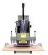
The Line Boring Machine is a power tool used to make multiple, quick, accurate, in-line holes in casework. To avoid accidents the following operational safety rules must be observed by everyone working on the GWG Line Boring Machine. Failure to be certified or to follow the safety rules will result in loss of shop privileges.
